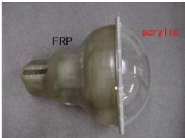
Figure 10: The acrylic cover and FRP case used from 2001 to protect the PMT from shock wave
