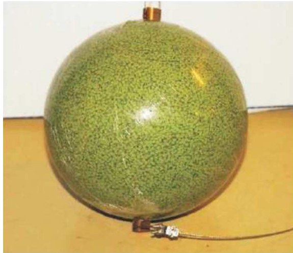
Figure 26: Ni ball used for relative Q.E. measurement [17]
