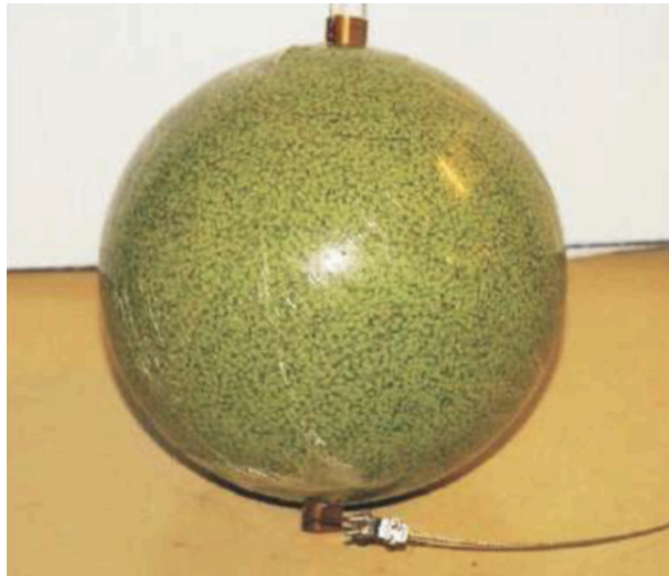
FIGURE 5.2: Appearance of the Ni-Cf source geometry. The figures are taken from [43].
