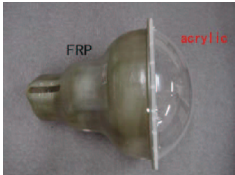
FIGURE 2.3: Image of the shockwave prevention case for 20-inch PMT
