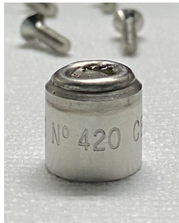
(A) Appearance of the AmBe source. (B) Appearance of the four pieces of BGO scintillator crystals.
