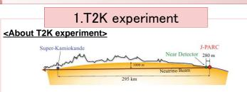
T2K(Tokai to Kamioka) is a long baseline neutrino oscillation experiment in Japan.T2K has observed  $v_{\mu} \rightarrow v_{e}$  or  $\overline{v_{\mu}} \rightarrow \overline{v_{e}}$  oscillation.  $v_{\mu}$  or  $\overline{v_{\mu}}$  beam is generated in J-PARC (Japan Proton Accelerator Research Complex) and go to SK(Super-Kamiokande). Neutrino beam is observed in J-PARC and SK , and check  $v_{\mu} \rightarrow v_e$  or  $\overline{v_{\mu}} \rightarrow \overline{v_e}$
