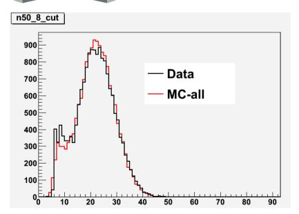
Neutron tagging with delayed coincidence
