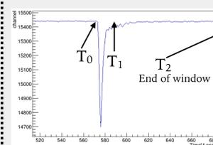
$$PSD \text{ par} = \frac{Q(T_2) - Q(T_1)}{Q(T_2)}$$
