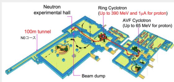
Proton beam was accelerated by two cyclotrons. Almost mono energetic neutron beam was produced through the  ${}^7\text{Li}(p, n){}^7\text{Be}$  reaction.
