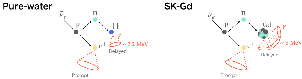
FIGURE 2.6: Idea of the delayed coincidence method for identification of inverse beta decay in pure-water phase (left) and SK-Gd (right).
